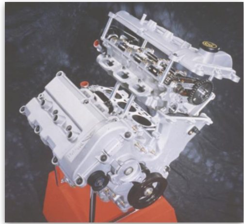
The 5 valve per cylinder Duratec
