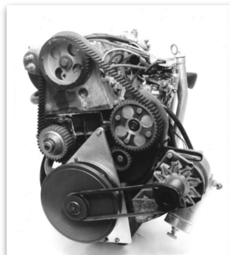
The contra rotating flywheel mounted on the front
